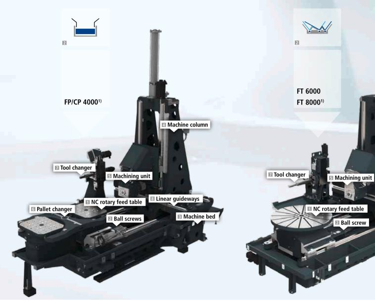
Every HELLER machine essentially comprises main components developed using FEM methodology. These include a machine bed optimised for stiffness and a mass-reduced column for high dynamics. At the same time, the vibration-optimised machine structure ensures the best surface quality during machining and long tool life.
